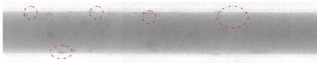
Fig. 10. Steel target rod with Zr cladding after exposure with protons in the target of the spallation source SINQ. The black points are attributed to the agglomeration of hydrogen on the inner side of the Zr cladding. Because the sample is highly activated, a well shielded facility was used for the investigations.
