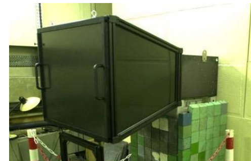
Scintillation plate (800 x 600 mm 2 ) Gadox Gd 2 O 2 S ; 1.5 mm
