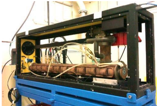
9 MeV LINAC (15 Gy/min at 1m)
