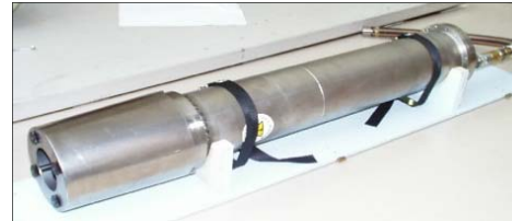
Pulsed DT neutron generator GENIE 36 SODERN, 2.10^9 n/s
